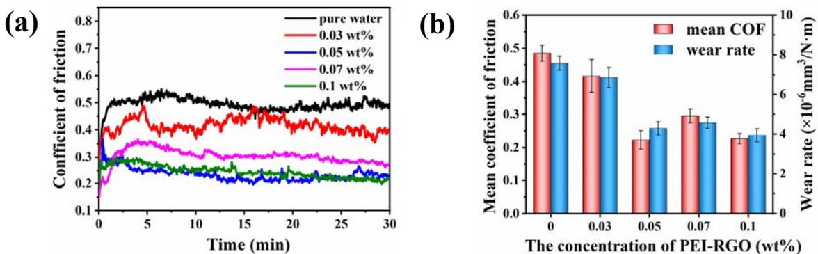
Figure 2. Tribological properties of water solution with different PEI-RGO mass fraction lubricated at frequency 3 Hz under 4 N load at ambient environment. (a) COF; (b) mean COF and wear rate.
