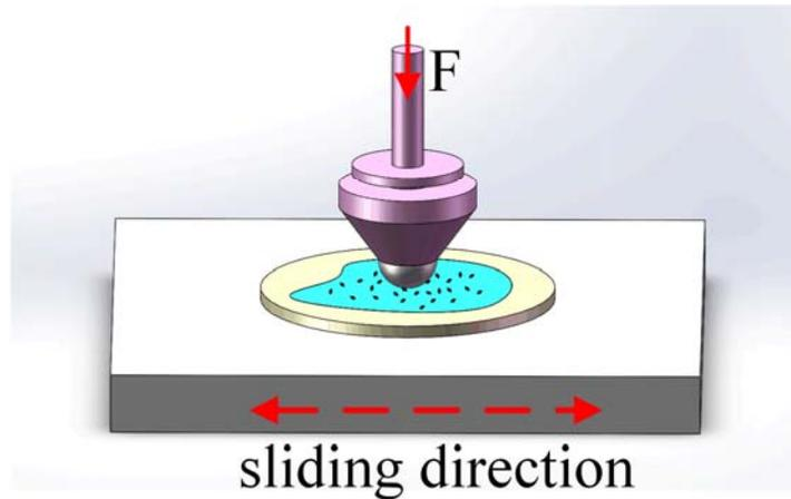
Figure 1. Schematic presentation of friction test.
